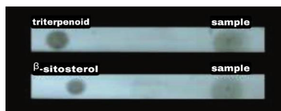
Figure 2. TLC chromatogram of the Binahong leaf extract showed that triterpenoid (lupeol) and \beta -sitosterol corresponded to the standard accordingly (Basyuni, Ginting, and Lesmana, 2017).
